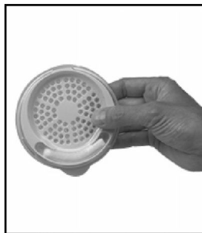
Figure 13. SimPlate for the quantification of heterotrophic plate counts in water. Reprinted with permission from IDEXX, SimPlate for HPC Unit Dose.
